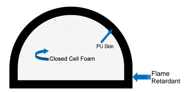
Supreme is the manufacturer of Polyurea (P.U.) Coated with closed cell foam fendering systems. Supreme Lightweight Foam Fender can be built in any shape and size with different dampening characteristics to fit the individual requirements of the vessel. It is spectacularly lighter and stronger than normal rubber fender, provides extra protection for the boat hull.
